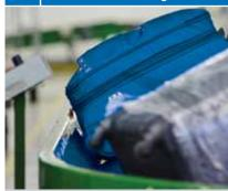
Belt conveyors transfer luggage, of varied shapes, to and around a corner in either a clockwise or counter-clockwise operation
