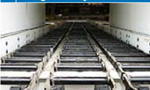
Drag conveyors can be used to meter or transfer bulk materials from one process to another. The design and characteristics of the drag conveyor enables it to fit almost any plant layout and is ideally suited to handle dry, free-flowing materials. A primary benefit of the drag conveyor include little product degradation during conveying and require less horsepower than other types of conveyors.
