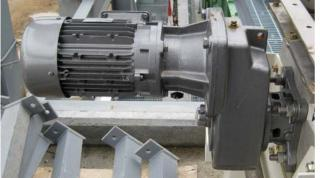
Screw Feeders are used to move bulk materials from silos, hoppers or bins. Screw Conveyors incorporate a screw rotating in a housing to transport the material. The bulk material flows forward with each revolution of the screw and is can be metered through the shroud for accuracy.
