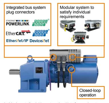
In this decentralized drive setup, signal interference is not an issue and long distances with screened cables are not required. The drives have safety functions on board and ensure direct communication between encoder and inverter (closed-loop operation). Additionally plug-and-work power and bus system connectors greatly simplify installation and maintenance. This saves time and expenses.
