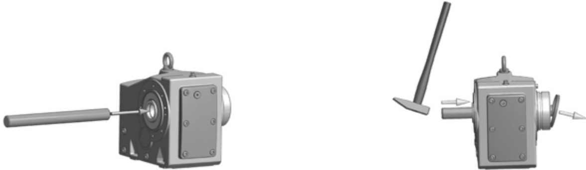
Figure 8: Removing the factory-fitted closing cap
