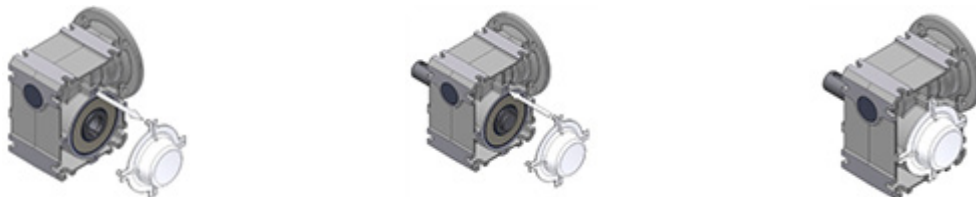
Figure 18: Removal and fitting of the cover cap
