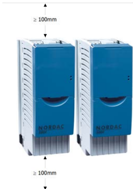
Fig. 1 Mounting distances for SK 5xxE
