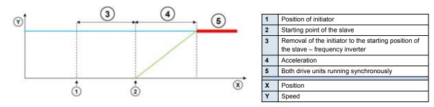
If the function is started, the slave frequency inverter accelerates to the speed of the master axis. The acceleration is specified via **ACCELERATION**. At low speeds the ramp is flatter and at high speeds there is a steep ramp for the slave frequency inverter. The acceleration path is stated in revolutions (1000 = 1,000 rev.) if P553 is specified as the setpoint position. If the setpoint position INC is used for P553, the acceleration path is specified in increments.
