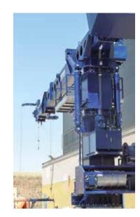
**Safe at any story.** – NORD drive technology gently moves the gondola and ensures precise positioning.
