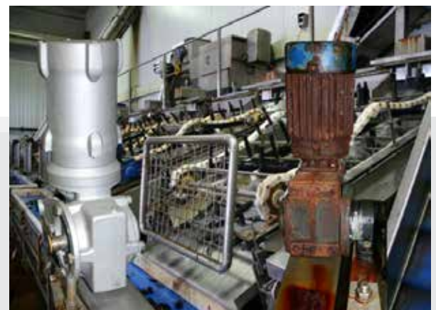
Resilient – a nsd tupH system (left) vs. a regular cast iron geared motor (right).
