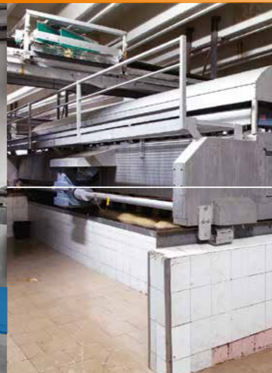
Malting plant turning machine with 14 drive units and travelling drive
