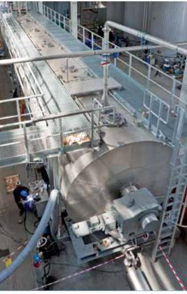
Powerful bevel geared motors mounted in pairs on the mixing drums deliver maximum output torques of over 53,000 Nm.
