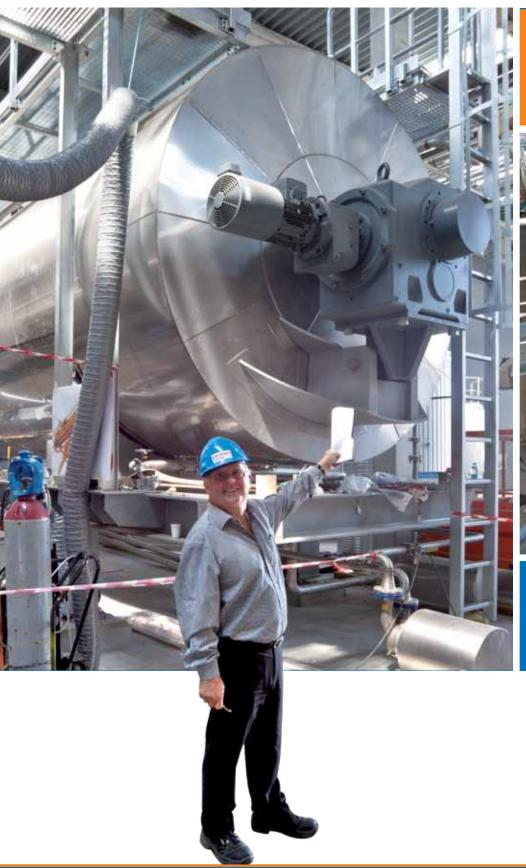
In four 20 m long mixing drums, movement is provided by bevel geared motors mounted in pairs on the longitudinal shaft.
