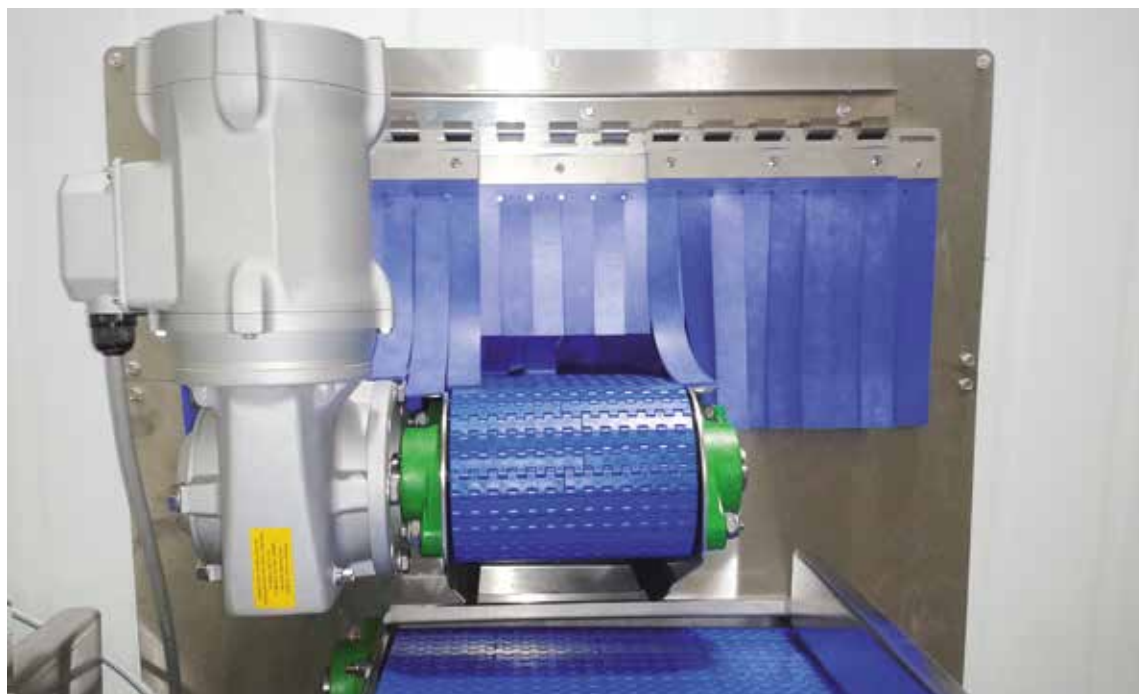
The nsd tupH surface treatment gives aluminum drives a smooth, permanently corrosion-resistant surface ideally suited to process industry applications.
