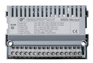
Compliance with the radio interference class C2 can only be ensured if the mains filter is active (jumper plugged into the upper position).
