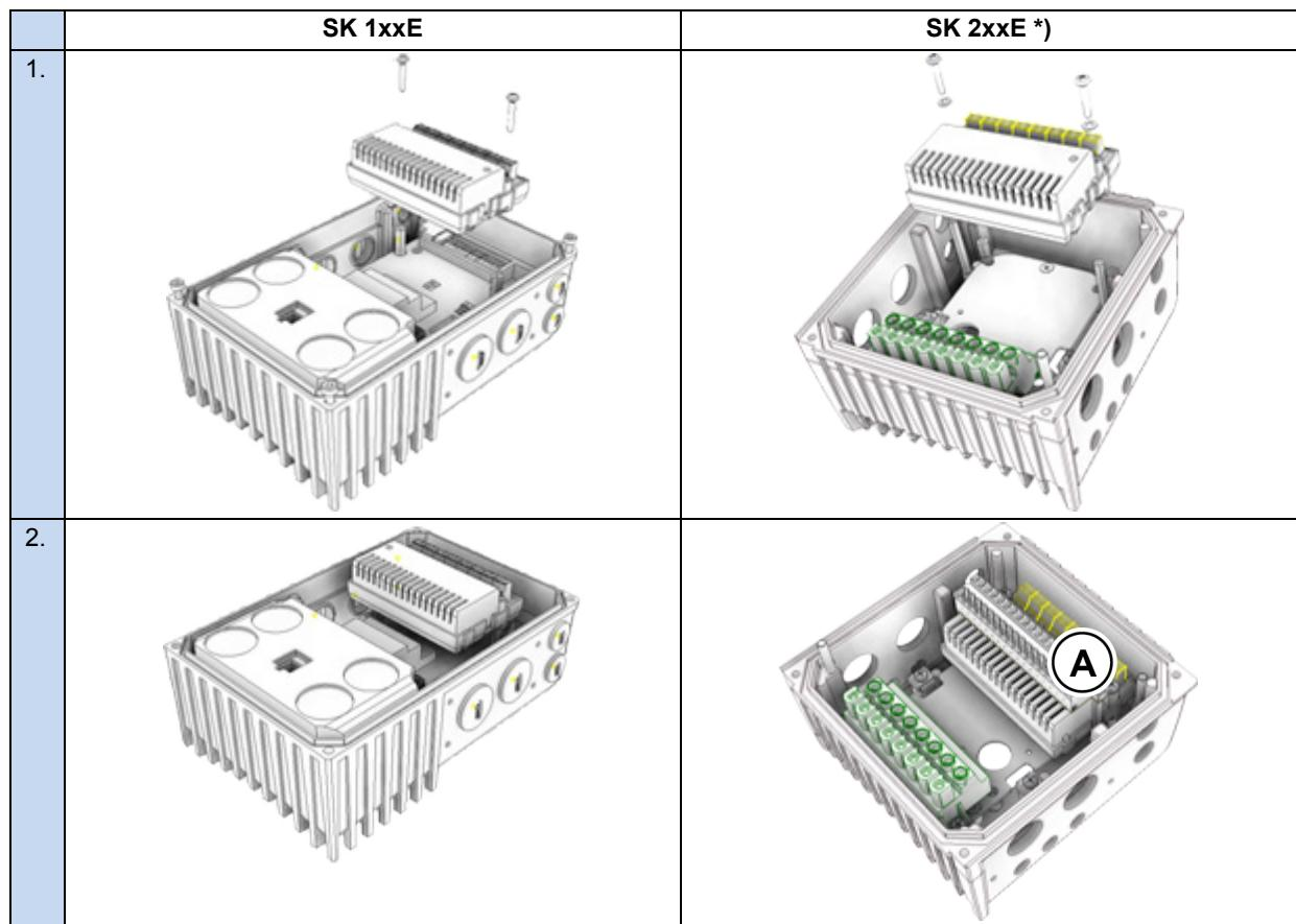
\*) Before carrying out installation step 1 it may be necessary to remove the control terminal bar (A).
