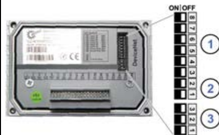
Factory settings DIP switches: OFF
