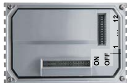
Factory settings DIP switches: OFF
