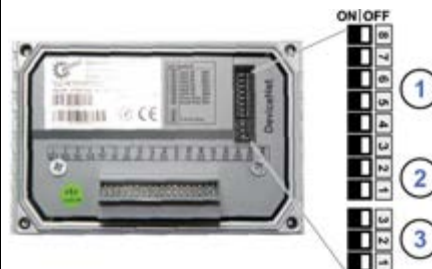
Factory settings DIP switches: OFF
