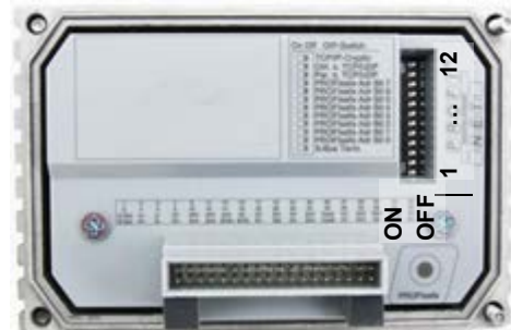
Factory settings DIP switches: OFF
