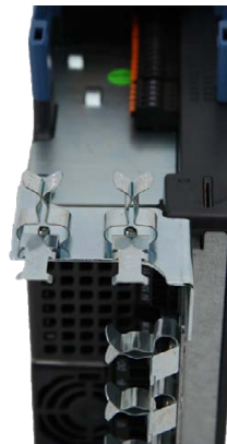
Detailed view of mounted EMC kits
