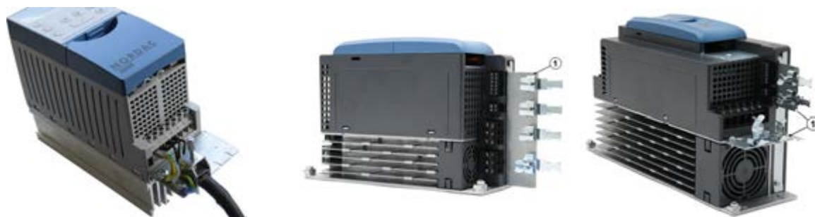
Figure 3: EMC kits installed for motor connection
